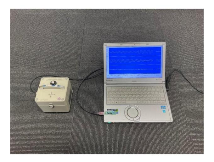
The photo shows microtremor sensor and laptop computer used in this study. Ambient vibrations observed by sensor are digitally recorded in computer through cable. The display of the computer shows three components of vibrations monitoring in real-time. Credit: Hiroyuki Miura, Hiroshima University
