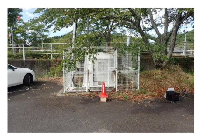
Ambient vibrations of ground are being recorded at a seismic observation station of Kyoshin Network (K-NET), a nation-wide strong-motion seismograph network in Japan since 1996. Seismograph is installed inside white cage. Credit: Hiroshima University
