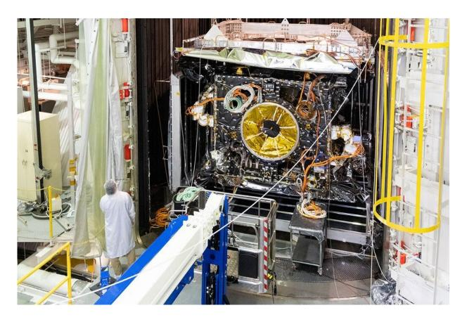
NASA's Psyche spacecraft is placed into the ultra-sturdy vacuum chamber at the agency's Jet Propulsion Laboratory in Southern California. Credit: NASA/JPL-Caltech
