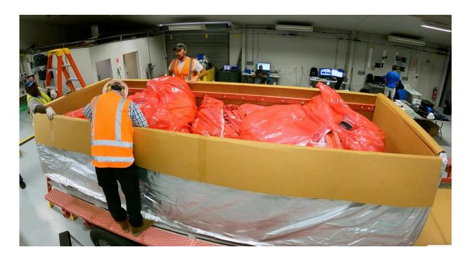
Technicians open a specialized shipping container with NASA's Super Pressure Balloon (SPB) in Wanaka, New Zealand, ahead of the 2022 launch campaign. The SPB is comprised of more than 10 acres of polyethylene film and weighs more than 5,300 pounds. Credit: NASA Wallops/Bill Rodman
