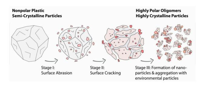
Process of the three-stage degradation of polyethylene particles. Within the environment, aggregation preferably occurs with natural colloidal systems. Credit: N. Meides, T. Menzel, A. Mauel.
