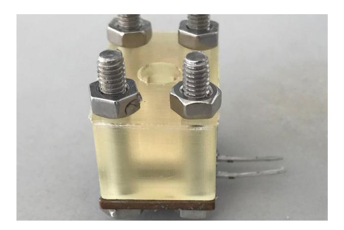
A 3D-printed device detects temperature changes when SARS-CoV-2 binds to molecularly imprinted polymer nanoparticles (ruler shows cm). Credit: Adapted from *ACS Sensors* 2022, DOI: 10.1021/acssensors.2c00100
