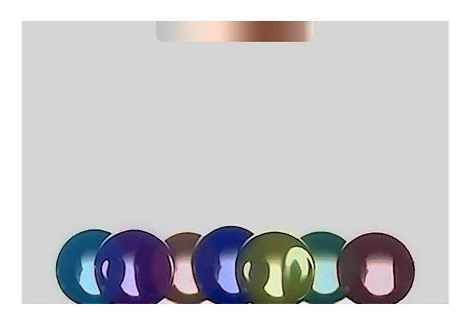
The DEST can move droplets with volume from tens of nanoliters to several milliliters and move droplets in an array. Credit: Jin Yuankai et al
