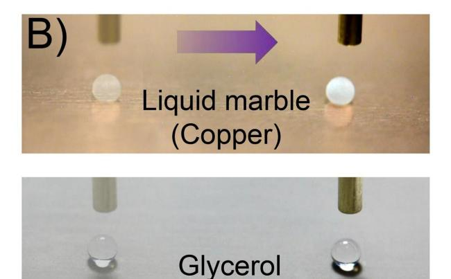
The DEST can move diverse types of droplets on electrically conductive substrates. Credit: Jin Yuankai et al/ DOI: 10.1073/pnas.2105459119
