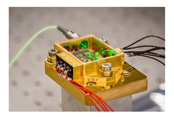
Small but mighty: The steady-state laser module constructed in Jena combines a tiny scale with great robustness. Credit: Fraunhofer IOF
