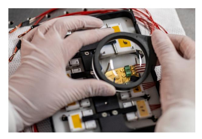
Raman spectrometer the size of a 50-cent piece. Credit: Fraunhofer IOF
