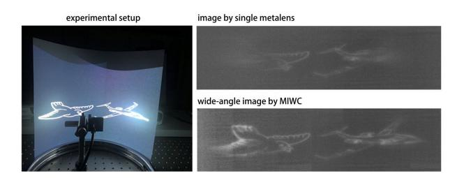
Researchers designed a new compact camera that acquires high-quality wideangle images using an array of metalenses. Their new planar camera (MIWC) produced clearer images of pictures projected across a curved screen compared to a camera based on a single traditional metalens. Credit: Tao Li, Nanjing University
