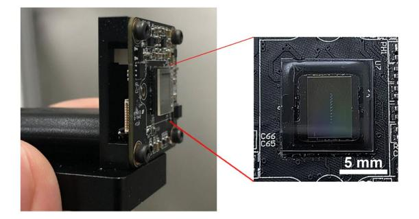
The researchers fabricated a metalens array (enlarged on the right) and mounted it directly to a CMOS sensor. This created a planar camera that measured about  $1 \text{ cm} \times 1 \text{ cm} \times 0.3 \text{ cm}$ . Credit: Tao Li, Nanjing University
