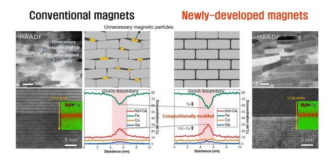
HAADF-STEM images and schematic illustrations of conventional magnets and newly developed magnets. Credit: Korea Institute of Materials Science (KIMS)
