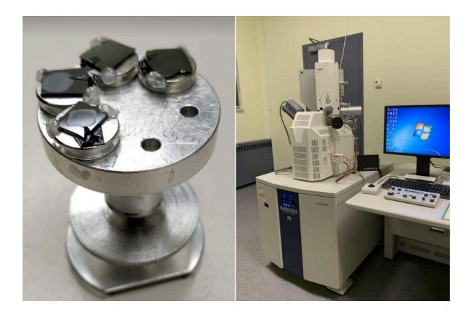
A scanning electron microscope (SEM) plate holding microplastic samples, left, and the SEM used for the project, right. Credit: Bin Shi
