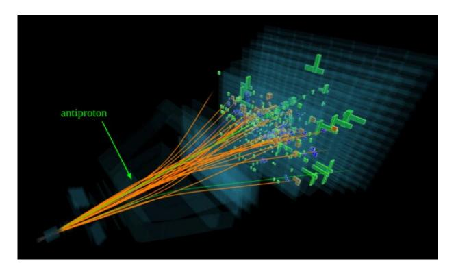
A proton–proton collision event recorded by the LHCb detector, showing the track followed by an antiproton formed in the collision. Credit: CERN
