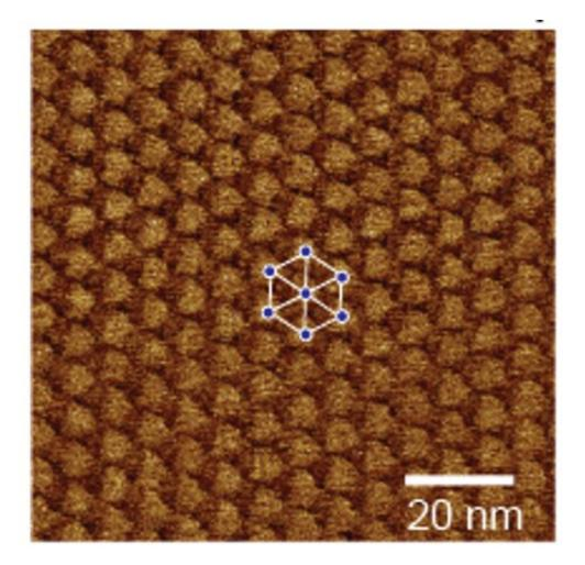
A top-view image, taken by piezoresponse force microscopy, of stacked layers of tungsten diselenide and tungsten disulfide, forming what is known as a heterostructure. Triangles indicate the repeating "units" of the moiré superlattice. Credit: Xi Wang/University of Washington
