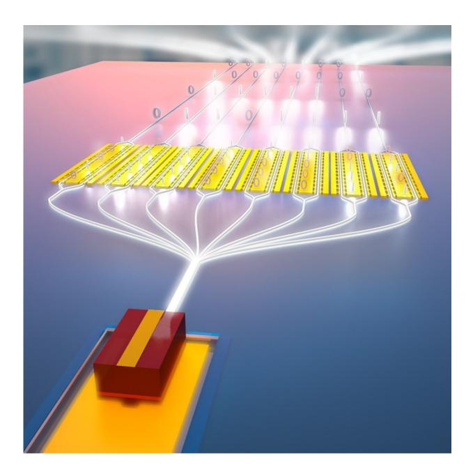
The on-chip laser is combined with a 50 gigahertz electro-optic modulator in
