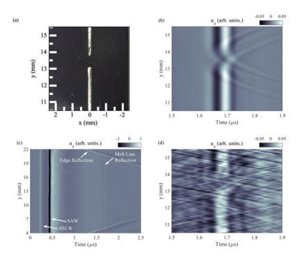
A Lawrence Livermore National Laboratory team demonstrated that a diagnostic incorporating surface acoustic waves—generated by laser-based ultrasound—could effectively and accurately evaluate laser melt lines and find defects in laser powder bed fusion metal 3D printing by scattering acoustic energy from melt lines, voids and surface features that can be quickly detected. Credit: David Stobbe/LLNL
