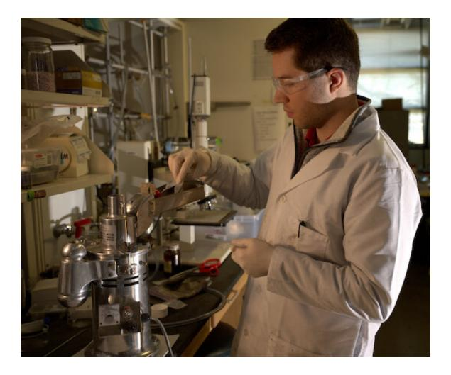
Graduate student Paul Savas feeds raw plastic into a crusher to prepare it for pyrolysis, or heating in an inert atmosphere. Credit: Jeff Fitlow, Rice University
