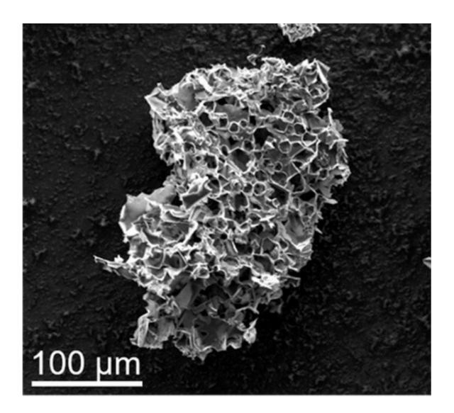
Pores in this micron-scale particle, the result of pyrolyzing in the presence of potassium acetate, are able to sequester carbon dioxide from streams of flue gas. Credit: Tour Group, Rice University
