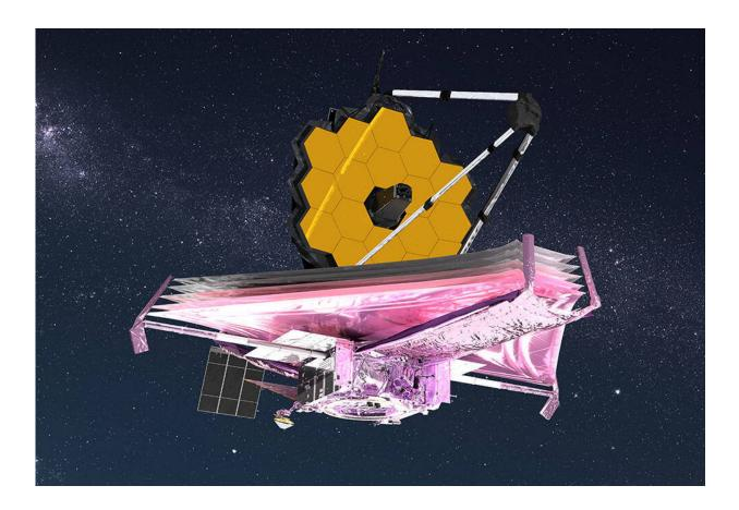
In this illustration, the multilayered sunshield on NASA's James Webb Space Telescope stretches out beneath the observatory's honeycomb mirror. The sunshield is the first step in cooling down Webb's infrared instruments, but the Mid-Infrared Instrument (MIRI) requires additional help to reach its operating temperature. Credit: NASA GSFC/CIL/Adriana Manrique Gutierrez
