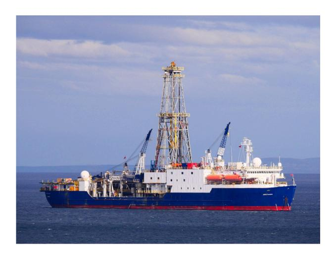
Drillship "JOIDES Resolution" with characteristic derrick. Credit: IODP
