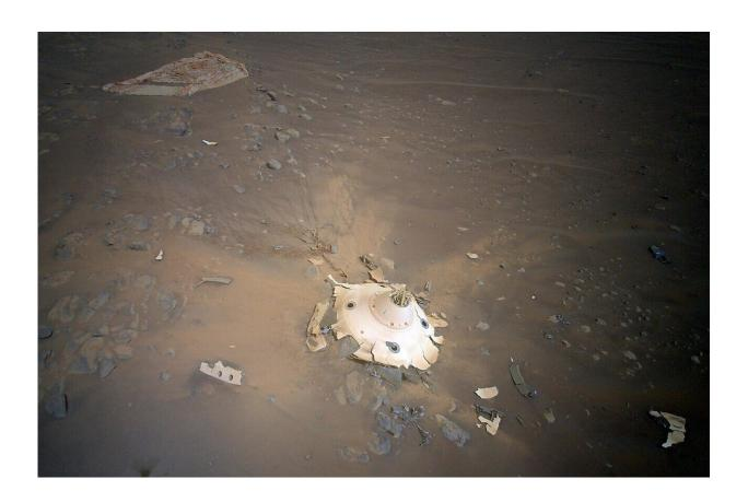
This image of Perseverance's backshell and parachute was collected by NASA's Ingenuity Mars Helicopter during its 26th flight on April 19, 2022. Credit: NASA/JPL-Caltech
