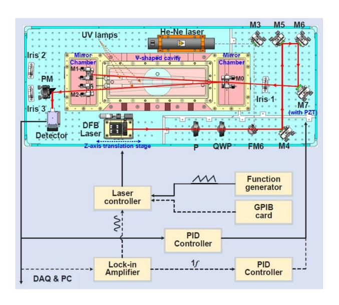
Schematic diagram of optical-feedback cavity-enhanced absorption spectroscopy
