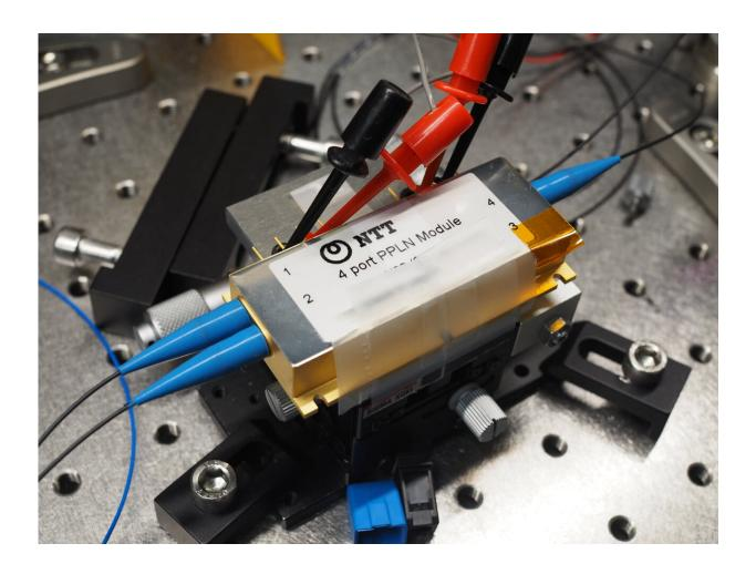
Researchers developed a new waveguide optical parametric amplifier (OPA) module (pictured), which they combined with a specially designed photon detector to generate strongly nonclassical light that can be used for quantum experiments. Credit: Kan Takase, University of Tokyo
