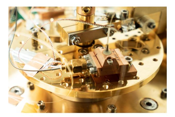
Researchers developed a new waveguide optical parametric amplifier (OPA) module, which they combined with a specially designed photon detector (pictured) to generate strongly nonclassical light that can be used for quantum experiments. Credit: Kan Takase, University of Tokyo
