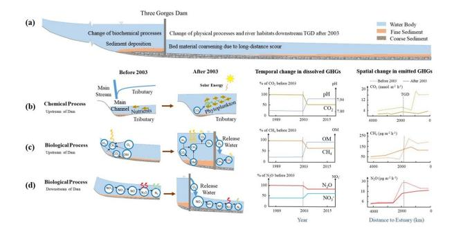
Whole system analysis concerning readjustment of physical and biogeochemical equilibria involved in regulation effects of the Three Gorges Dam on GHGs emissions from the Yangtze River, China. Credit: Science China Press
