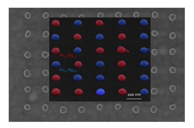
This electron microscopy image of nanostructures shows nanostructures with different proportions of gold (Au) and silver (Ag) in different colors. Credit: EPFL
