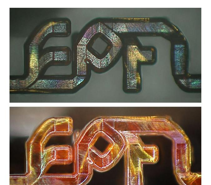
The team also fabricated the EPFL logo to show how that the method can be used to make complex 3D shapes. The top image shows dark-field illumination, and the bottom shows bright-field illumination. Credit: Yves Bellouard, Ecole Polytechnique Fédérale de Lausanne
