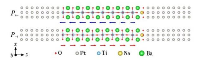
The schematic diagrams of the atomic structures in the left and right polarization states of NaTi-FTJ. Credit: Xiao Wei
