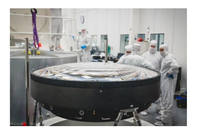
Optical lens for the Large Synoptic Survey Telescope (LSST). Credit: Farrin Abbott/SLAC National Accelerator Laboratory
