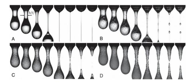
A droplet of silicone oil pinches of from fluids with different concentrations of 140 µm particles: (A) is pure liquid, (B) is 2% concentration, (C) is 20%, and (D) is 50%. Credit: Thiévenaz and Sauret
