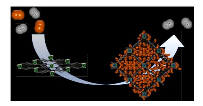
Only deuterium can open the pores of DUT-8, while hydrogen leaves the framework closed. This highly selective detection leads to a high separation selectivity combined with high deuterium uptake. Credit: Dr. Volodymyr Bon
