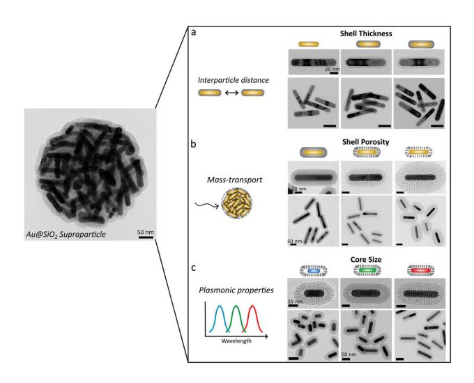
Silica-coated AuNR supraparticles as a tunable platform for sensing: the interparticle distance, mass- and heat-transport and plasmonic properties can all be tuned via the properties of the individual Au@SiO<sub>2</sub> NR building blocks. Credit: *Advanced Functional Materials* (2022). DOI: 10.1002/adfm.202200148
