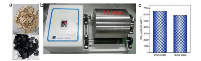
Large-scale carbon hydrogasification. a) Pinewood, and as-prepared charcoal after wood pyrolysis. b) Home-made roll-mill with a 15-liter container. c) Comparison between small-scale planetary mill and large-scale roll-mill.
