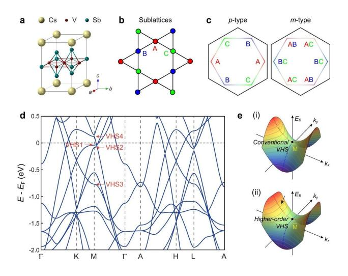
a) The Lattice structure of kagome metals CsV<sub>3</sub>Sb<sub>5</sub>. b) Real space structure of the kagome vanadium planes. The red, blue, and green coloring indicate the three kagome sublattices. c) Two distinct types of sublattice decorated van Hove
