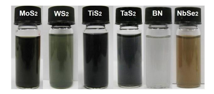
TMD nanosheets the team obtained are solution-processable and printable. Credit: *Nature Protocols* (2022). DOI: 10.1038/s41596-021-00643-w
