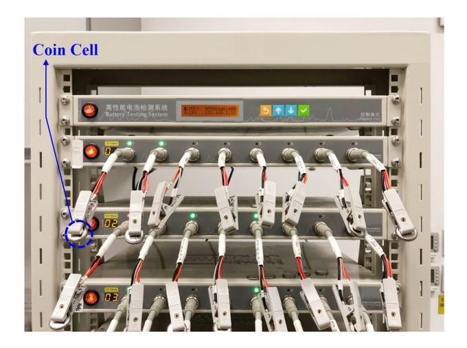
By using this battery testing system, the amount of intercalated lithium ions in layered materials can be controlled effectively by tuning the cutoff voltage. Credit: *Nature Protocols* (2022). DOI: 10.1038/s41596-021-00643-w
