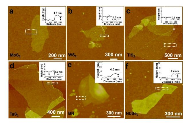
Images of the exfoliated nanosheets of a, MoS2. b, WS2. c, TiS2. d, TaS2. e, BN. f, NbSe2. Mono- and few-layer inorganic nanosheets were successfully produced by this method. Credit: *Nature Protocols* (2022). DOI: 10.1038/s41596-021-00643-w
