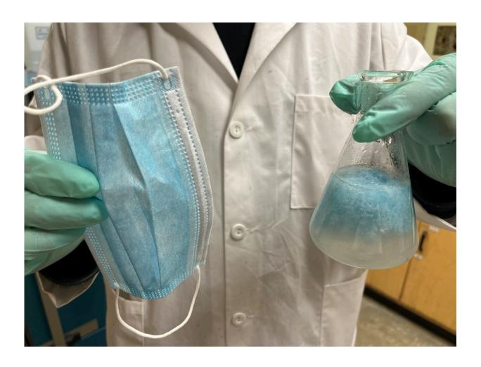
The WSU researchers developed a process to fabricate tiny mask fibers, ranging from five to 30 millimeters in length, and then added them to cement concrete to strengthen it and to prevent its cracking. Credit: WSU
