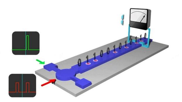
Schematic illustration of skyrmions based racetrack memory device. Credit: WEI Wensen
