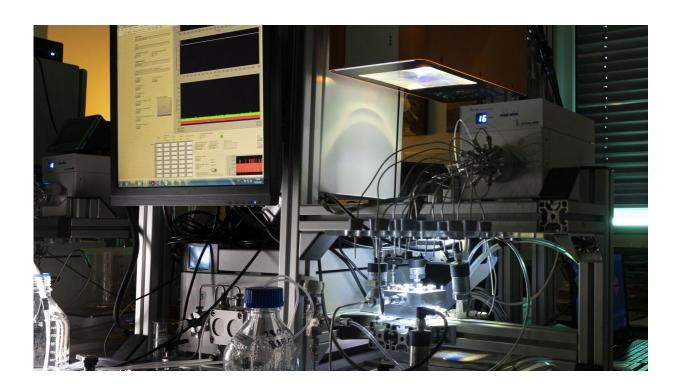
Photocatalytic membrane filtration system with a sun simulator. The membranes are coated with titanium dioxide. Credit: Markus Breig, KIT
