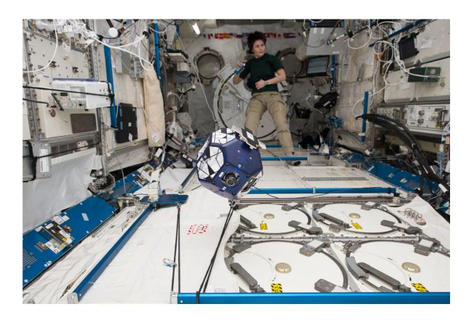
ESA (European Space Agency) astronaut Samantha Cristoforetti conducts a test run for SPHERES during her previous mission to the space station in 2014. For that investigation, students wrote software to direct multiple free-flying satellites in creating 3D models of a target object. Credit: NASA
