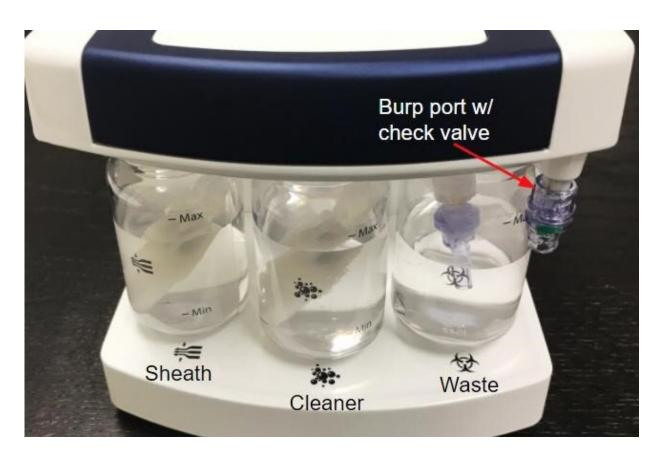
This preflight view of rHEALTH ONE hardware shows fluid bottles used in the experiment operations without the custom bags required for the bottles to function in microgravity. Credit: rHEALTH
