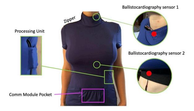
This image shows the components of the Smart-Shirt garment, including integrated sensors, wiring, and a communication module to transmit scientific data via a wireless link for BEAT experiment, part of the Wireless Compose-2 investigation. The technology demonstration builds on work by the German Space Agency (DLR) to develop wireless network infrastructure to support scientific experiments on the space station. Credit: DLR
