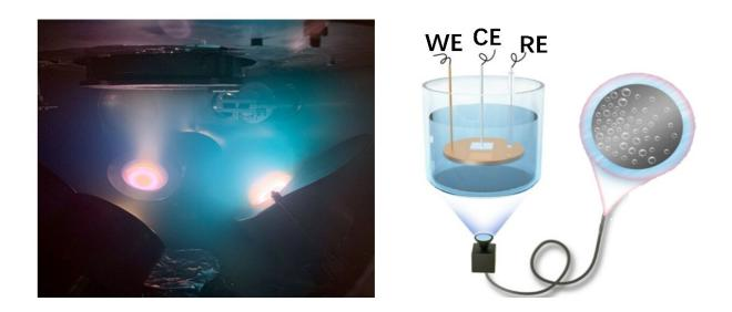
Schematic illustration of high-throughput bubble screening method. Credit: NIMTE
