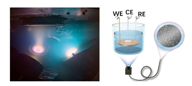
Schematic illustration of high-throughput bubble screening method. Credit: NIMTE
