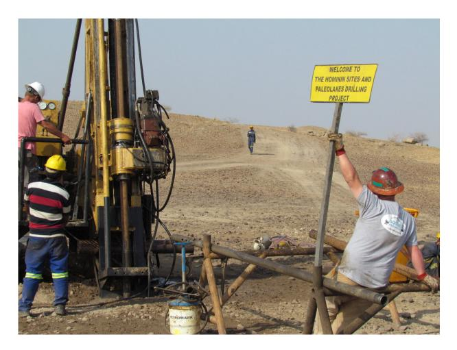
Workers use a drilling rig to collect samples of lake sediments from deep underground. Credit: Andrew Cohen/University of Arizona
