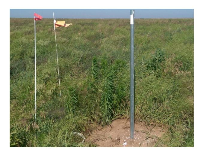
Soil greenhouse gas monitoring chamber, mid-season. The photo was taken at a native tallgrass prairie site at Grazinglands Research Laboratory in El Reno, Oklahoma. The study focused on monitoring three major greenhouse gas sources – carbon dioxide, methane, and nitrous oxide. Credit: Brekke Munks
