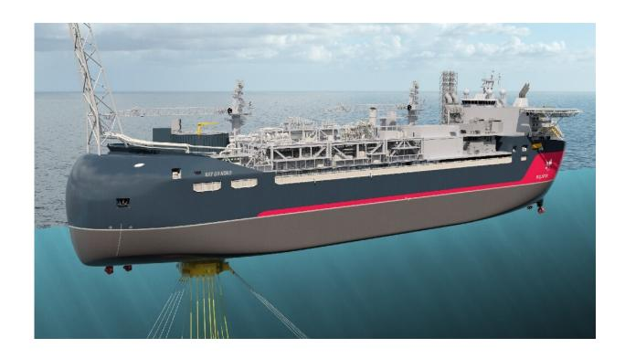
An illustration of the planned Bay du Nord Floating Production Storage and Offloading (FPSO) vessel.
