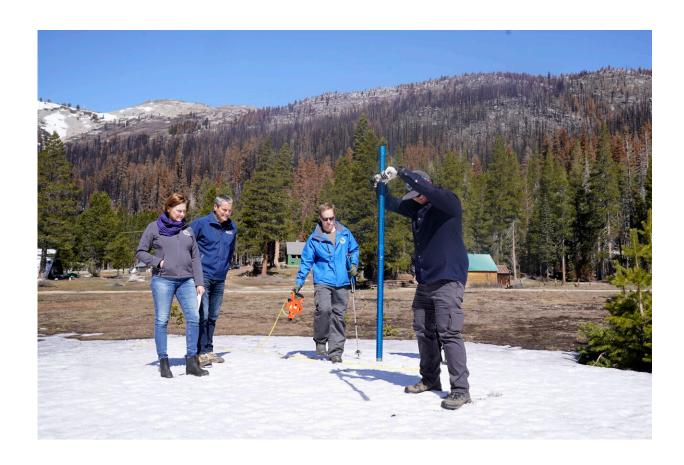
Sean de Guzman, manager of snow surveys and water supply for the California Department of Water Resources, plunges the snowpack measuring tube into a small patch of snow on the snow course as he conducts the fourth snow survey of
