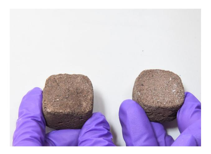
Space bricks developed from Martian soil simulant using slurry-casting method. Credit: Nitin Gupta
