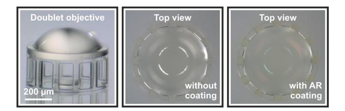
Researchers developed a new way to apply anti-reflective coatings to 3D-printed multi-lens systems such as the doublet objective pictured here, which is just 600 microns in diameter. These coatings help minimize light losses due to reflection, which is critical for making high-quality 3D printed systems consisting of multiple microlenses. Credit: Simon Ristok, University of Stuttgart
