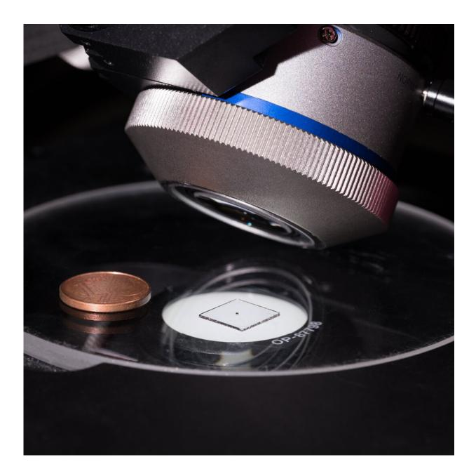
The researchers used a microscope to acquire tilted-view images of a 600-micron-diameter doublet lens system 3D printed on a  $1x1 \text{ cm}^2$  glass slide. The doublet lens system is visible as the small dot in the center of the glass slide. The coin is included for scale. Credit: Moritz Flöss, University of Stuttgart
