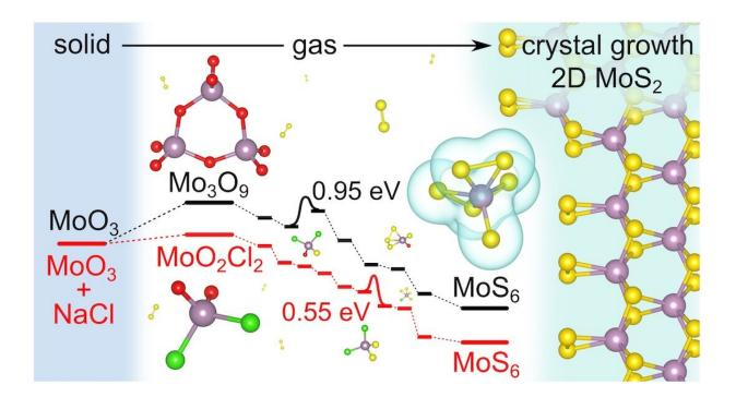
Common salt (NaCl) acts as an intermediary in the chemical vapor deposition growth of 2D molybdenum disulfide, speeding the process of its creation. Materials theorists at Rice University discovered that salt and a precursor form a eutectic, which has a lower melting temperature than either of them. Credit: Jincheng Lei/Yakobson Research Group
