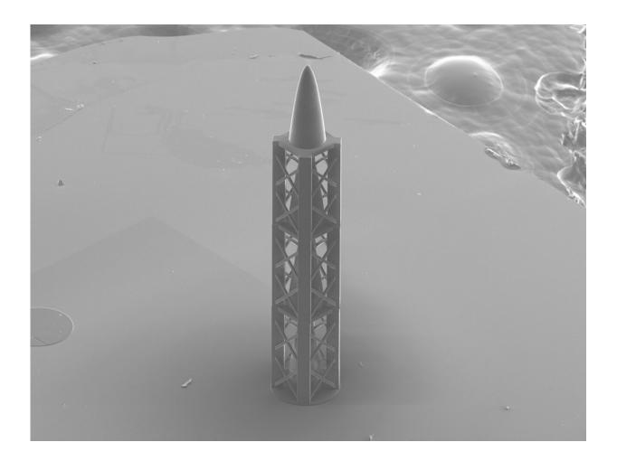
A microstructure created by a 3D printer: the innovative refractive structure developed by PSI scientists and which combined with a diffractive element, results in an achromatic X-ray lens, is almost a millimetre long (or high, as shown in the photo). Turned on its end, it resembles a miniature rocket. It was created by a 3D printer using a special type of polymer. This image of the structure was captured using a scanning electron microscope. Credit: Paul
