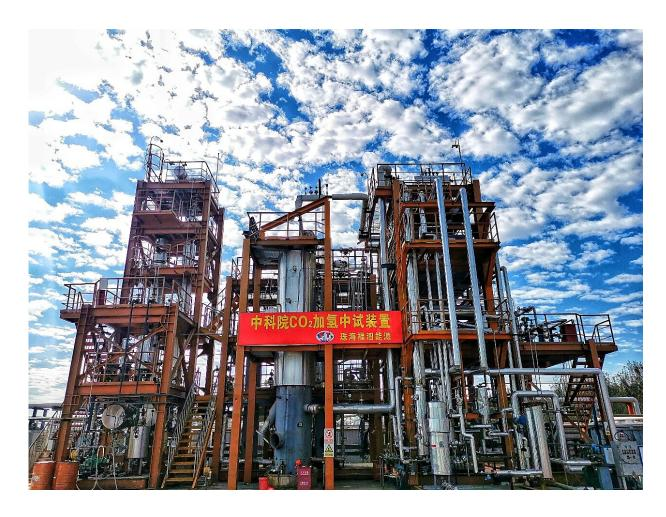
The world's first demonstration device for 1,000 tons/year production of gasoline from carbon dioxide hydrogenation has completed its trial operation and technology assessment on March 4. Credit: DICP
