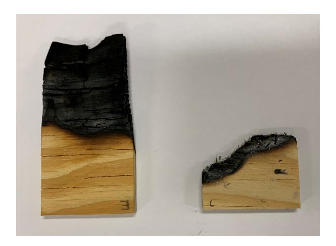
Coated wood (left) can resist flames, limiting fire damage, unlike bare wood (right). Credit: Ethan Iverson
