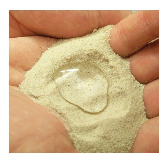
Paraffin wax-coated sand is an extremely water-repellant material, which keeps
