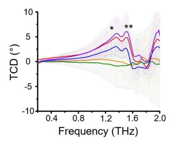
This graph shows the terahertz circular dichroism spectra of five different brands of 1-carnosine. While three samples show the same pattern of peaks, the measurement suggests possible differences from the remaining two samples. Credit: Wonjin Choi, Kotov Lab, University of Michigan
