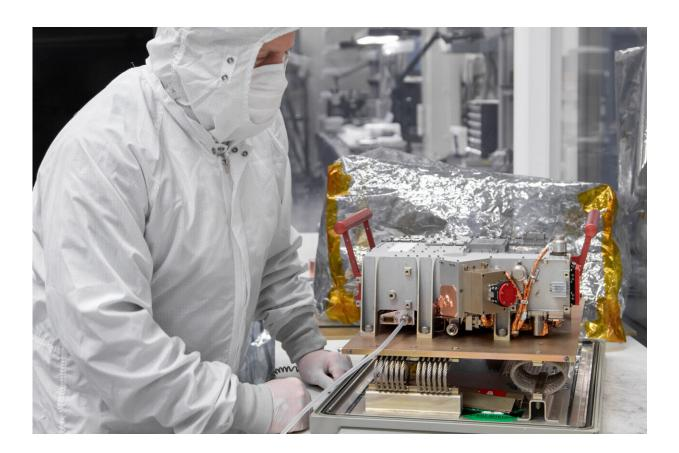
Southwest Research Institute's Ultraviolet Spectrograph (UVS) was the first instrument delivered for integration into NASA's Europa Clipper spacecraft. The instrument collects ultraviolet light to study the composition of the atmospheric gasses and surface materials of Europa, one of Jupiter's largest moons with a suspected subsurface ocean. Credit: SwRI
