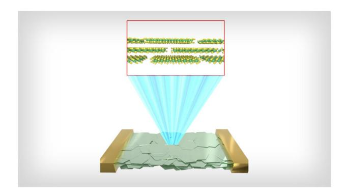
The layered patchwork design of van der Waals thin films enables the membrane to stretch and flex over irregular geometries. Credit: Yan et al./UCLA
